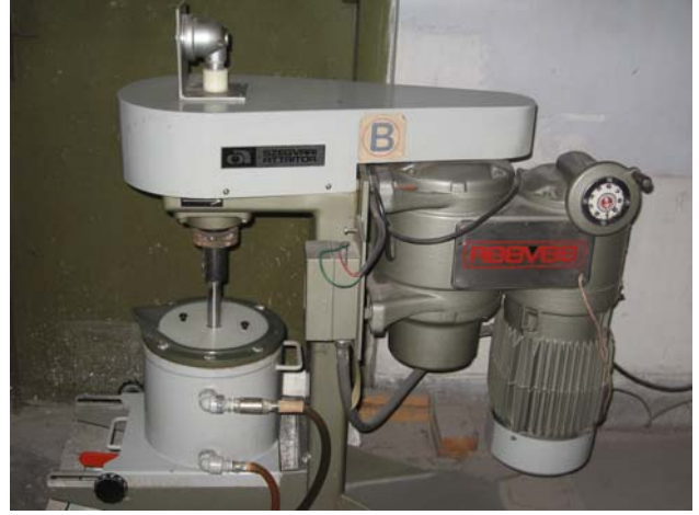
Attritor Mill, Union Process, USA Capacity: 7.5 litre
