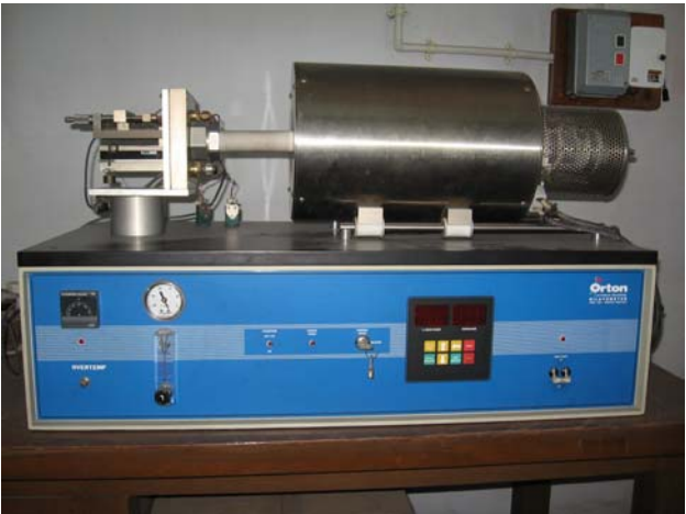
High Temperature Dilatometer Orton, USA Temperature: upto 1600°C
