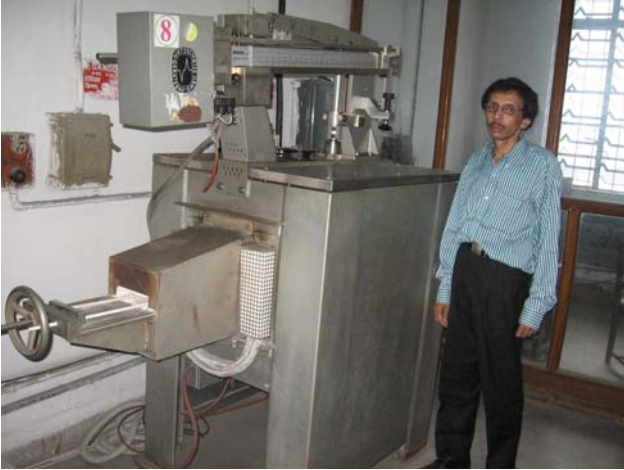
Hot MOR, Netzsch, Germany Temperature: 1400°C
