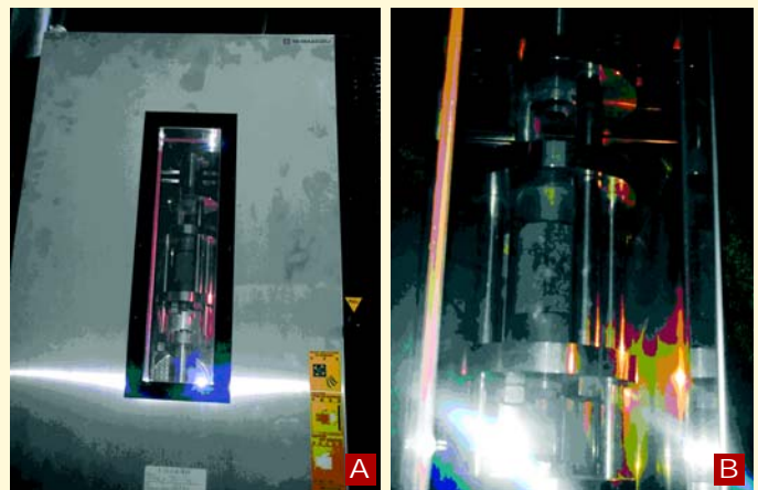
Fig. 5: Testing of repair mortars at higher temperature (a) Thermostatic chamber (b) Compression test specimen inside the thermostatic chamber
