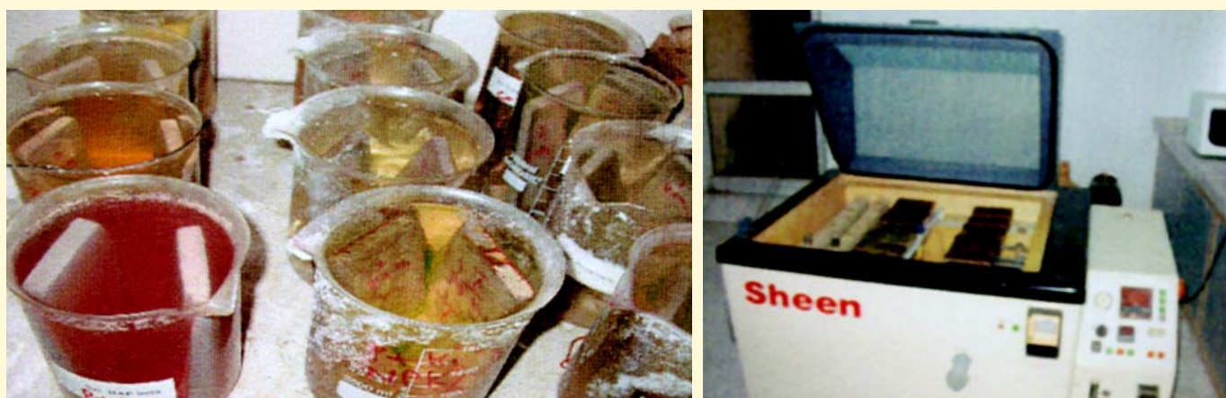
Fig. 8: Coated panels with developed formulations under test
