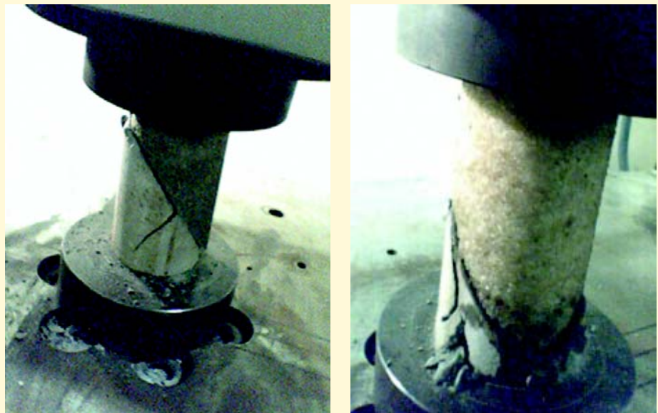
Fig. 3: Polymer modified Repair Material under Test
