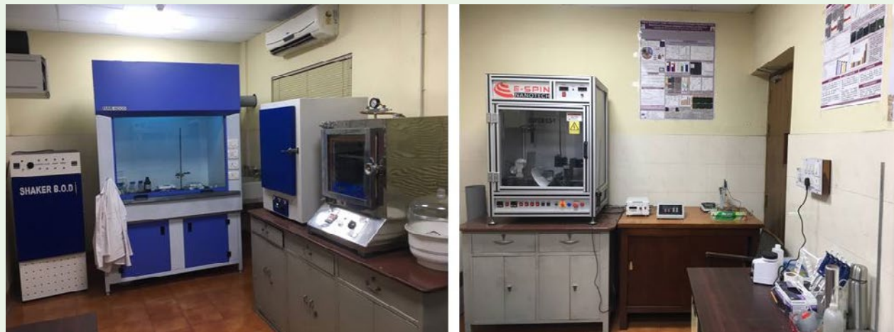
Electropolishing equipment (Super ES-1), fume hood, BOD incubator and others
