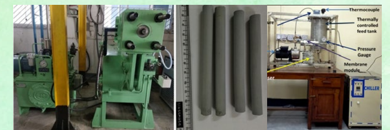
Hydraulic extrusion press of 20 ton capacity and Membrane Distillation setup
