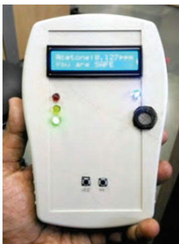
(a) Fabricated handheld device, and (b) Comparison of device results with GC-MS.
