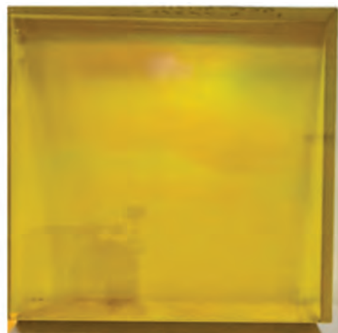
Coated RSW Glass block (dimension: 400 x 400 x 100mm 3 )
