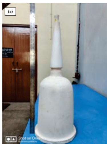
Bottom pouring refractory pot with dent tube; and RSW glass casting through bottom pouring refractory pot
