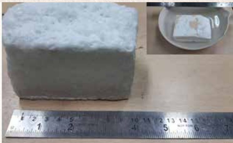
Light weight porous foam glass brick of size 50 X 70 X 100 mm 3 developed at CGCRI (Inset: Foam glass is floating on water)
