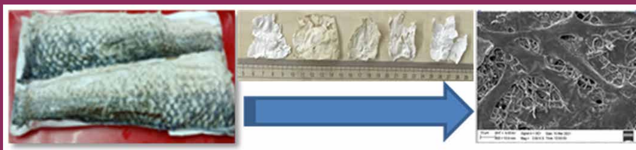
Isolation of collagen from Rohu skin (Labiorohita) and the fiber mat derived from it (right)
