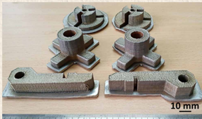
Photograph of demonstration parts of 8620 steel parts made using DED
