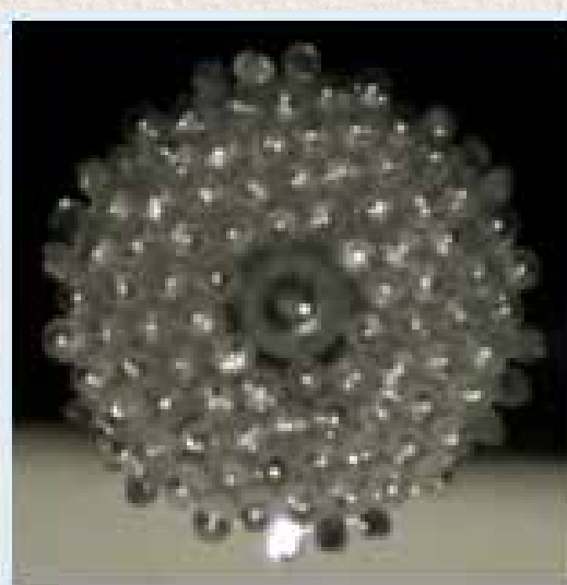
Stack of capillaries (left). The seven central capillaries are replaced by a single capillary in case of PBG fiber stack (right)
