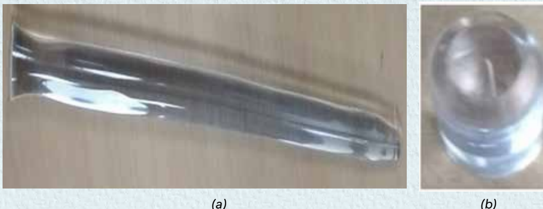
Axial (a) and radial (b) view of Ca and Mn assisted Cr^{+4} doped nano-engineered yttria-alumina-silica (YAS) glass based optical fiber preform
