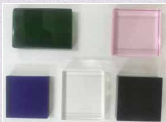
The images of different colored, transparent and sealing (black) glasses produced using quartz extracted from fly ash
