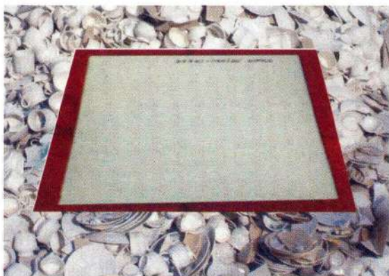
Ceramic tiles engobe developed using fired crockery and sanitaryware scraps
