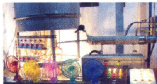
10-cell SOFC stack and its demonstration
