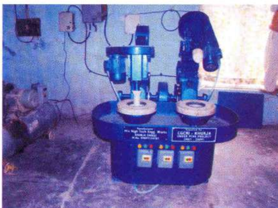
Indigenously developed Roller Head Jigger Machine at Outreach center, Khurja
