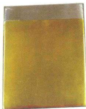
Ag-doped hard-coating (coated area ~10x10cm 2 ) on stainless steel substrates
