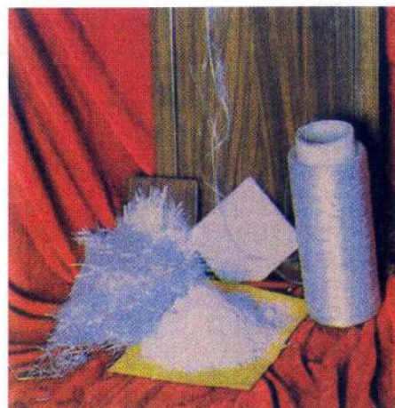
Raw materials for making GRG boards, finished and unfinished products
