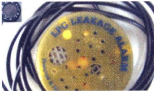
Gas Leakage Alarm (inset: Sensor Head)
