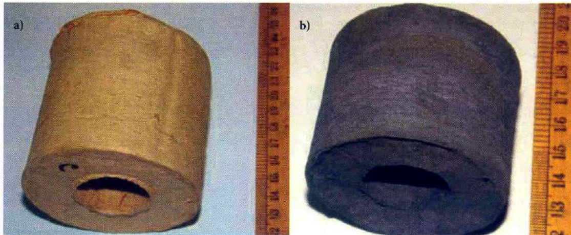
Porous tubular SiC using cellulosic material: (a) as-cast pulp fiber tubes and (b) porous SiC tube made thereof
