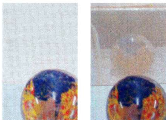
Image of the paperweight on a) Uncoated tile and b) Sol-gel coated tile showing coatings capable of imparting colour and improving gloss of developed glazed tiles
