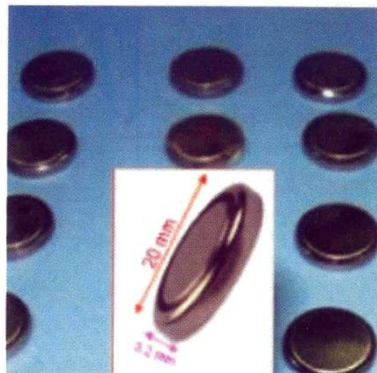
Fabricated 2032 type Li-ion coin cells using oxide cathode and anode
