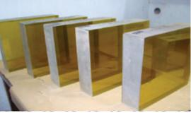
Bottom-Pouring-Flow-Casting and Radiation Shielding Window (RSW) Glass blocks
