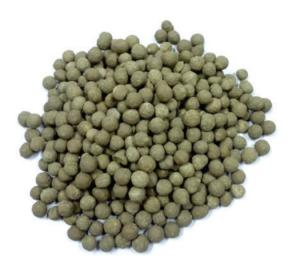
Sintered mullite aggregates form bauxite
