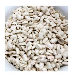
Synthetic Magnesium aluminate spinel aggregate
