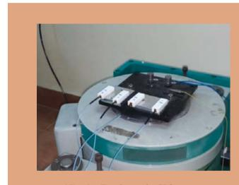
Vibration Test Set up for FBG sensors
