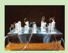
Laboratory setup for testing trace (2-50 ppm) moisture in transformer oil
