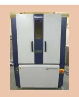
X-ray diffractometer (Ultima IV, Rigaku, Japan)
