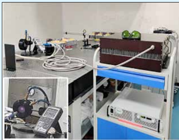
CSIR-CGCRI-made 300 W CW Yb Fiber Laser Module
