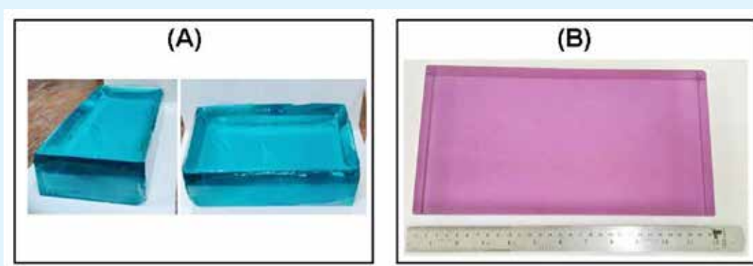
(A) Annealed clad glass blocks and (B) Nd-doped laser glass block of size 310x165x45mm 3
