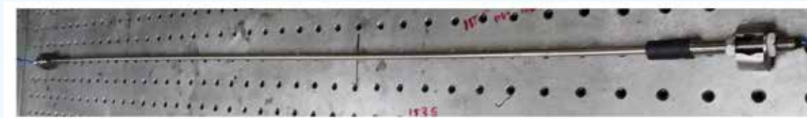
Developed long gauge fiber Bragg grating strain sensor
