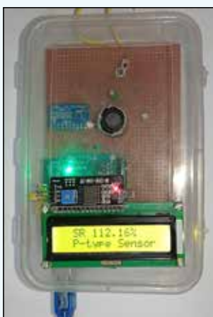
A lab-level prototype for the detection of trace formalin adulteration in fish
