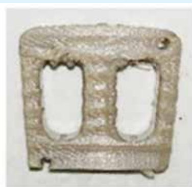
Spinal cage implant prototype for spinal inter-body fusion surgery applications
