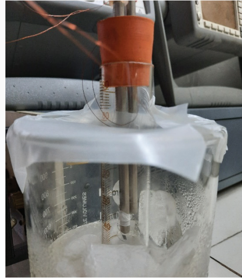
Flat sensor for in-situ ammonia sensing Low temperature ammonia sensing set-up
