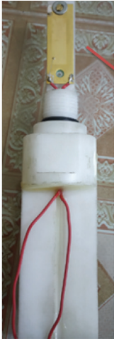
Sensor dip in transformer oil with data transmitter system
