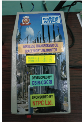
Sensor data receiver system from transformer (500 m)
