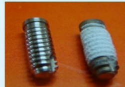
Plasma spray HAp coated dental implant
