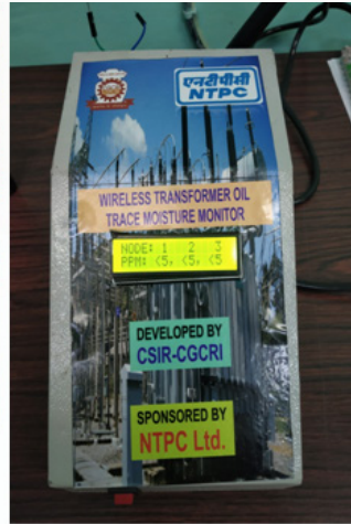
Sensor data receiver system from transformer (500 m)
