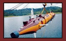
Underwater Vehicle (UV-150) for seabed mapping, coastal surveillance etc
