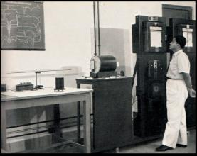
A set-up for Differential Thermal Analysis of clay minerals.
