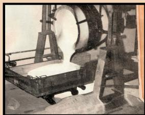
Casting of optical glass slabs.
