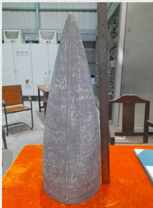
Size-B Radome 249.6 mm (Base OD) X 633 mm (Height)
