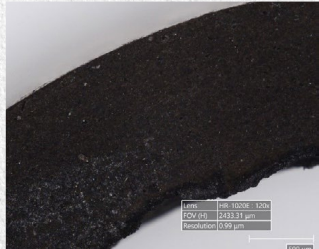
Ceramic support coated with functionalized coating solution
