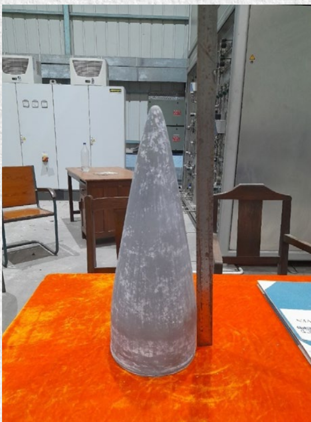
Size-A Radome 178 mm (Base OD) X 471.5 mm (Height)
