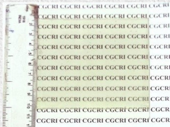
2 Electrode Electrochromic Assembly on 10cm x10 cm ITO glass
