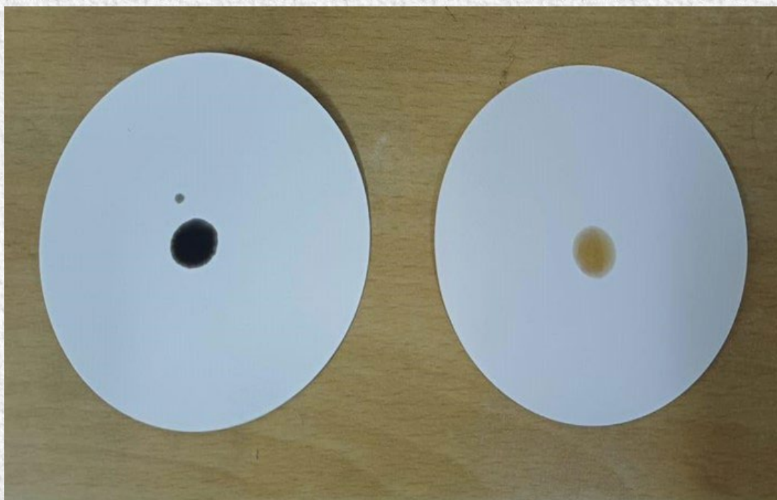
Drop test of waste engine oil and membrane permeated oil
