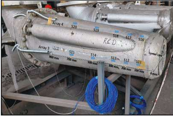
Side view of Instrumented blowpipe showing two arrays of sensors and GUI developed for critical temperature prediction of Blowpipe
