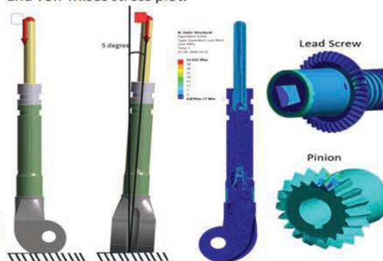
(c) Finite element model with Boundary condition and von-Mises stress plot.
