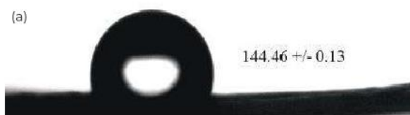
Water contact angles of NIPS films (a) untreated and (b) treated with 2.5M KOH
