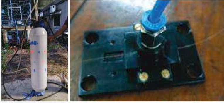
In figure, (a) Array of 12 fiber Bragg gratings tested on the liner of type IV cylinder and (b) developed fiber optic and electronic (resistive) hydrogen sensors
