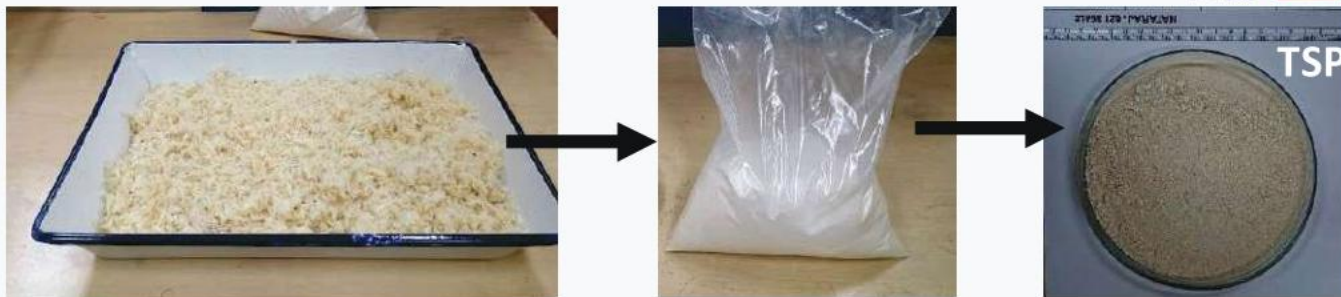
Phosphoric acid treatment on fish scale derived inorganic substance to develop triple super phosphate (TSP). Preparation of 1 Kg batch
