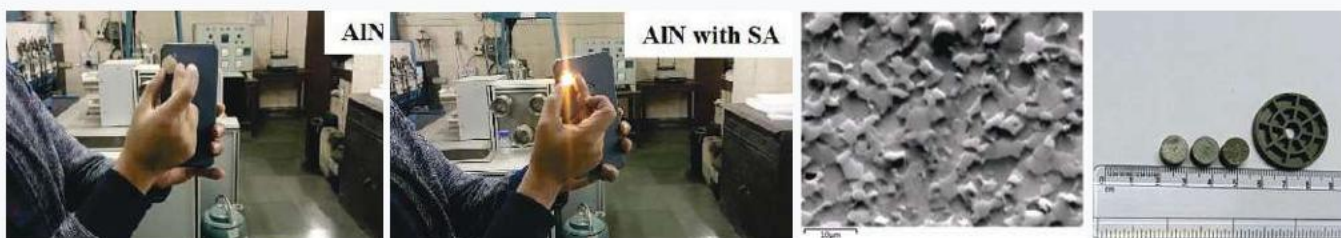
Spark plasma sintered AlN ceramics a) Pure b) with additive c) Microstructure
