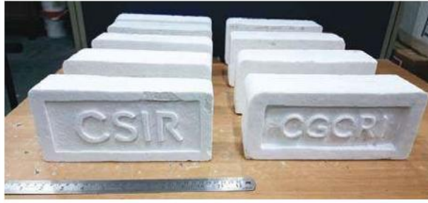
Lightweight porous glass foam bricks developed using glass waste (Dimension: 240 x 110 x 70 in mm)
