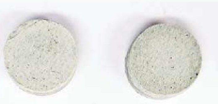
MgAlON ceramics prepared at 1600°C carbothermal reduction nitridation route.
