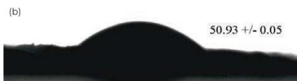
Water contact angles of NIPS films (a) untreated and (b) treated with 2.5M KOH
