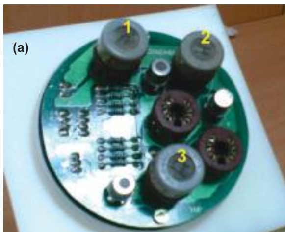
(a) Array of CGCRI-made sensors in an e-nose [1. \text{SnO}_2\text{-Sr} (5 wt%), 2. \text{SnO}_2\text{-Ba} (5 wt%), 3. \text{SnO}_2\text{-Ag} (1 wt%)]
