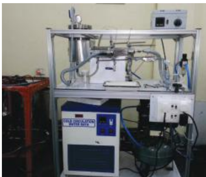
CSIR-CGCRI developed ceramic hydrophobic membrane based MD setup
