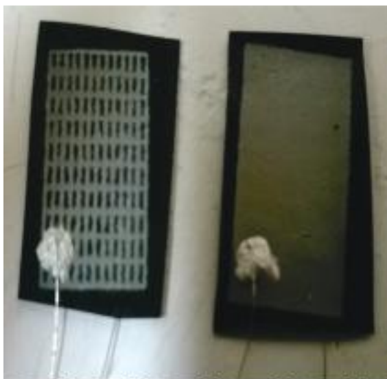
Fullerene dispersed -alumina humidity sensor
