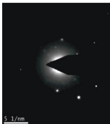
TEM images of (L) Antacid particles showing self assembled structure and (b) SAD pattern exhibiting characteristic polycrystallinity
