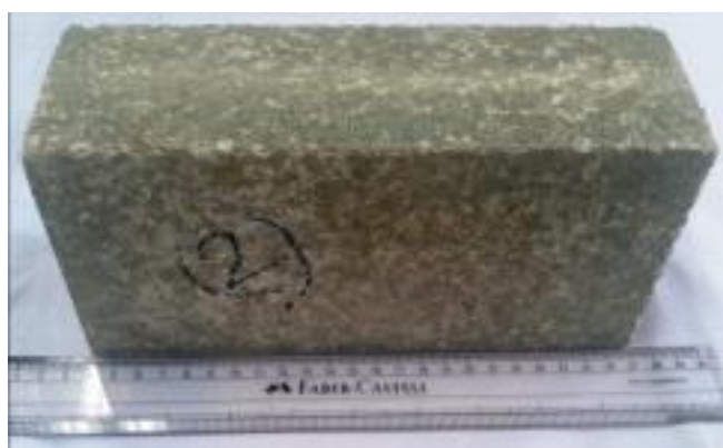
30% alumina containing standard size brick developed using insulator waste
