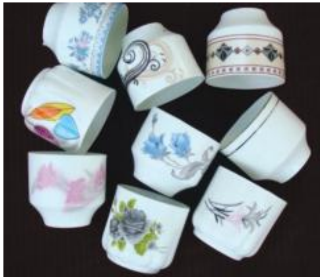
Low maturing bone china tablewares developed utilizing dicalcium
