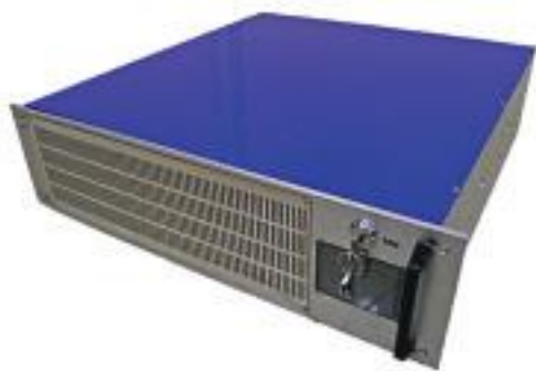
Prototype of 10W Tm-fiber laser module under packaging
