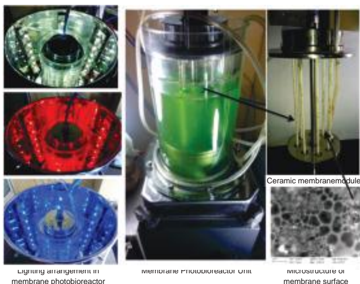
Lab-scale membrane photobioreactor for algal biomass production
