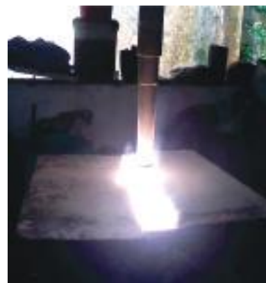
Plasma fusion of CSIR-CGRI refractory samples
