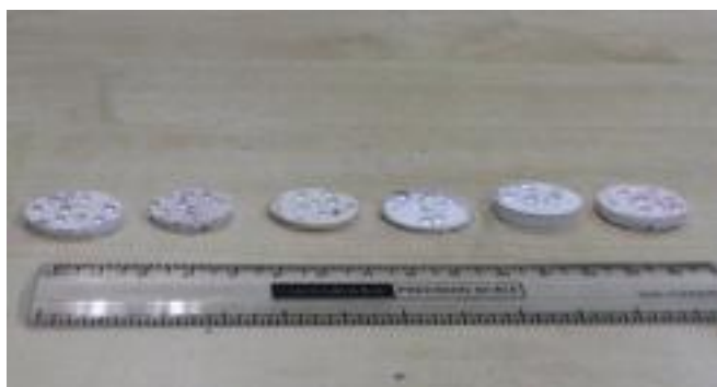
CSIR-CGCRI developed ceramic hydrophobic disc membrane
