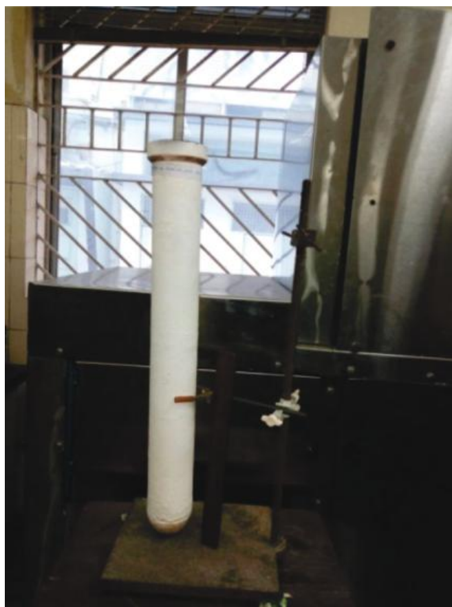
Mullite membrane coating on SiC for hot gas filtration
