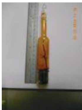
(L) As prepared chalcogenide glasses in sealed silica ampule and (R) Transmission spectrum of an as prepared chalcogenide glass
