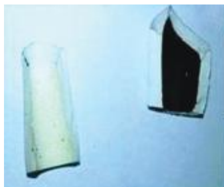
Photograph of DDR zeolite membrane layer (a) without carbon and (b) with carbon membrane
