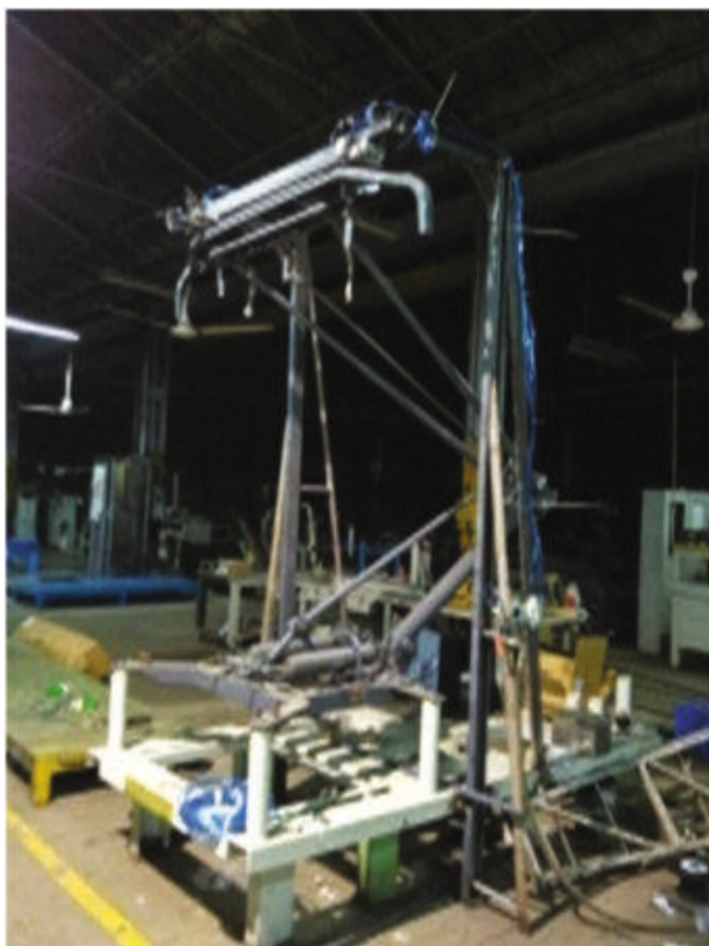
Test bed for evaluation of optical strain sensors for measurement of contact force and contact location
