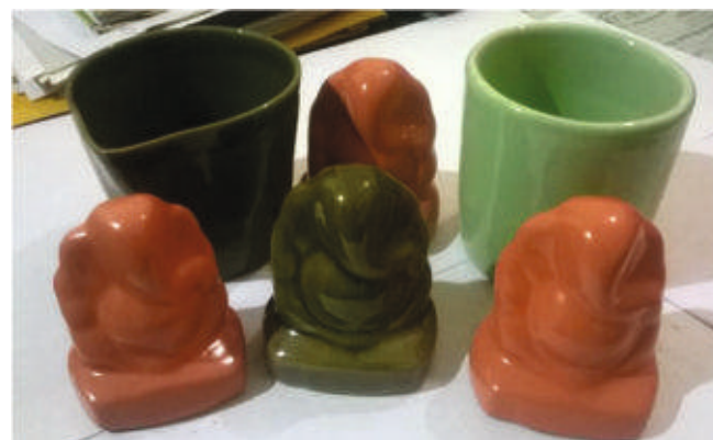
Glazed Stoneware Products using Fly Ash in the range of 20 – 35%
