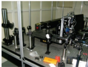
FBG sensor fabrication system
