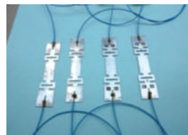
Packaged FBG strain and temperature sensors
