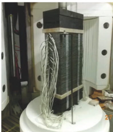
1kW SOFC Stack fabricated and demonstrated at CSIR-CGCRI wherein the developed sealant has been used as one of the components
