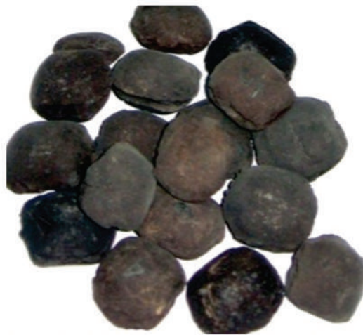
Sintered Mag-chrome aggregates produced at a refractory plant
