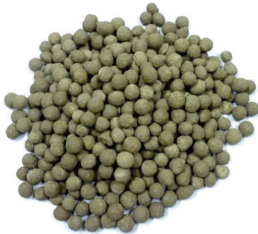
Sintered mullite aggregates form bauxite
