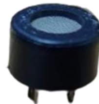
Fig.1. (a) Diabetes breath analysis criteria, and (b) packaged diabetic sensor module.
